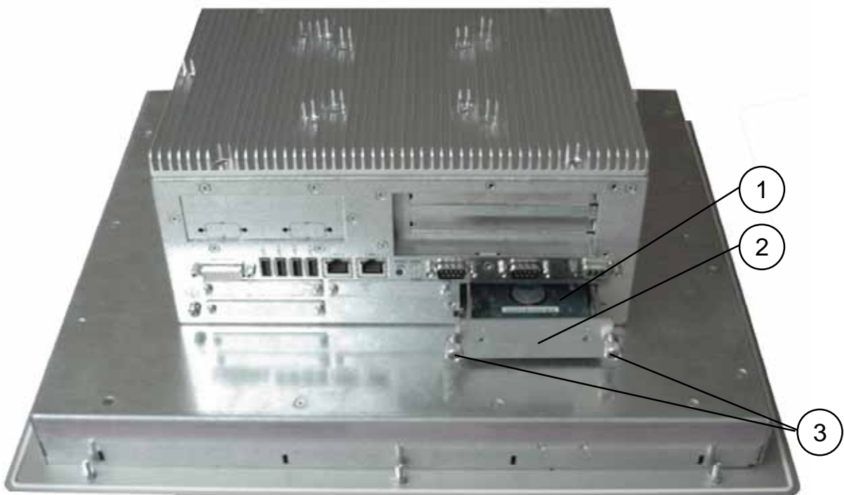
Fig. 6: Bottom side of V Panel Express (shown with opened removable drive cage)
