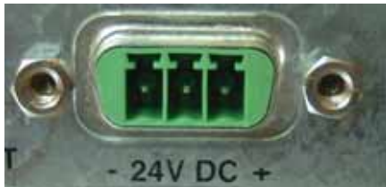
Fig. 10: DC-connector (without Phoenix plug terminal)
