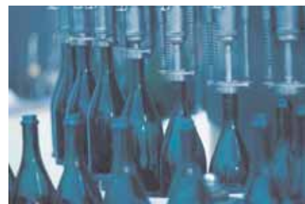
Automatic bottle shutting with torque limiting
