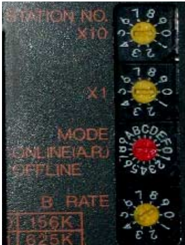
Figure 5.2.1-1 Rotary Switches of the Master Station
