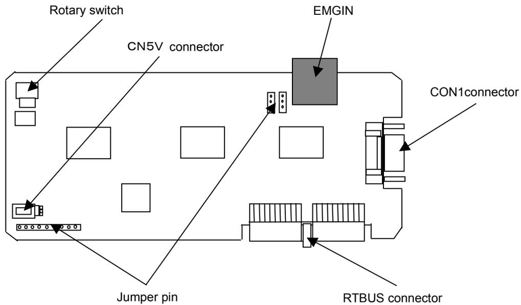
Fig. 9.1.1 Additional axis interface card general drawing
