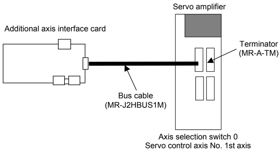
Fig. 8.7.2 Connection of controller and servo amplifier
