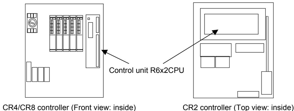
Fig. 5.3.1 Control unit R6x2CPU position in the controller
