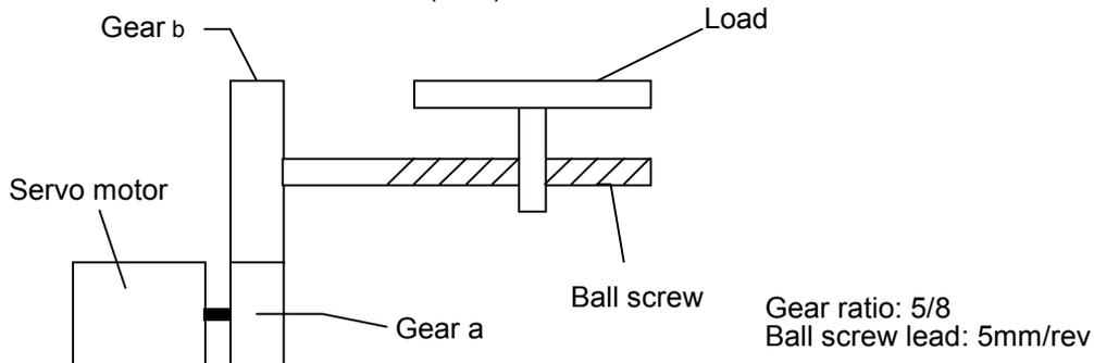
Fig. 7.1.2 Inside of direct moving unit
