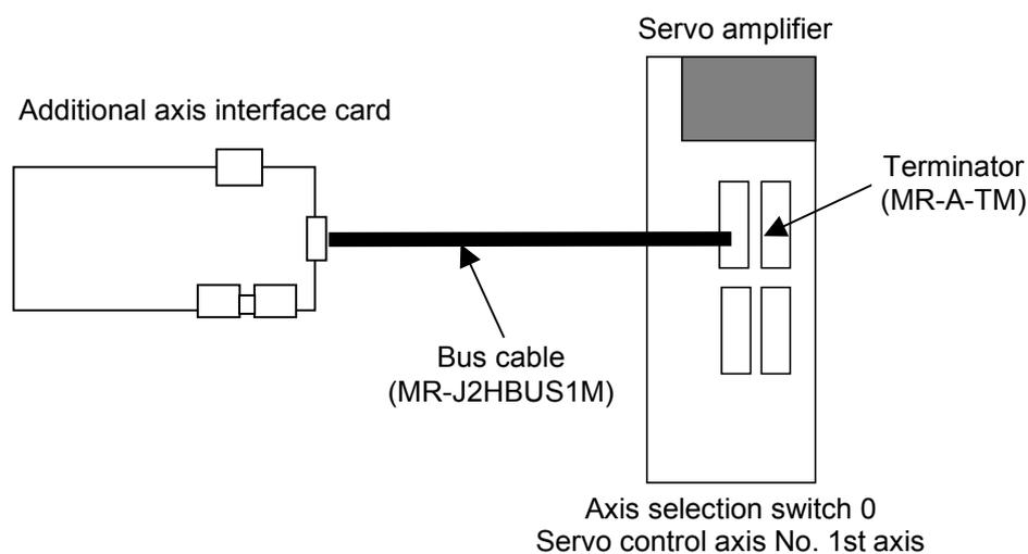
Fig. 7.6.2 Connection of controller and servo amplifier
