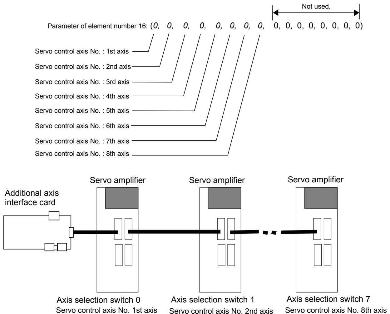
Fig. 8.2.1 Control No. and parameter element of servo
