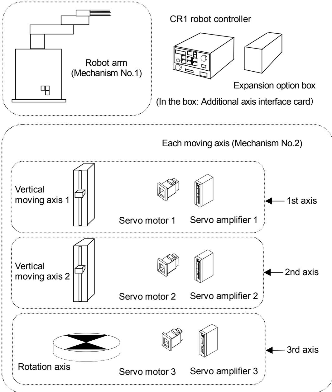
Fig. 8.7.4 System with multiple axes
