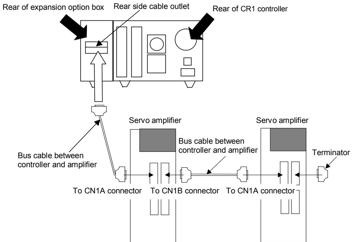
Fig. 5.1.3 Connection of CR1 controller and servo amplifier
