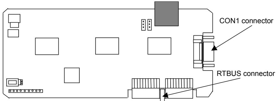
Fig. 5.1.2 Additional axis interface card general drawing
