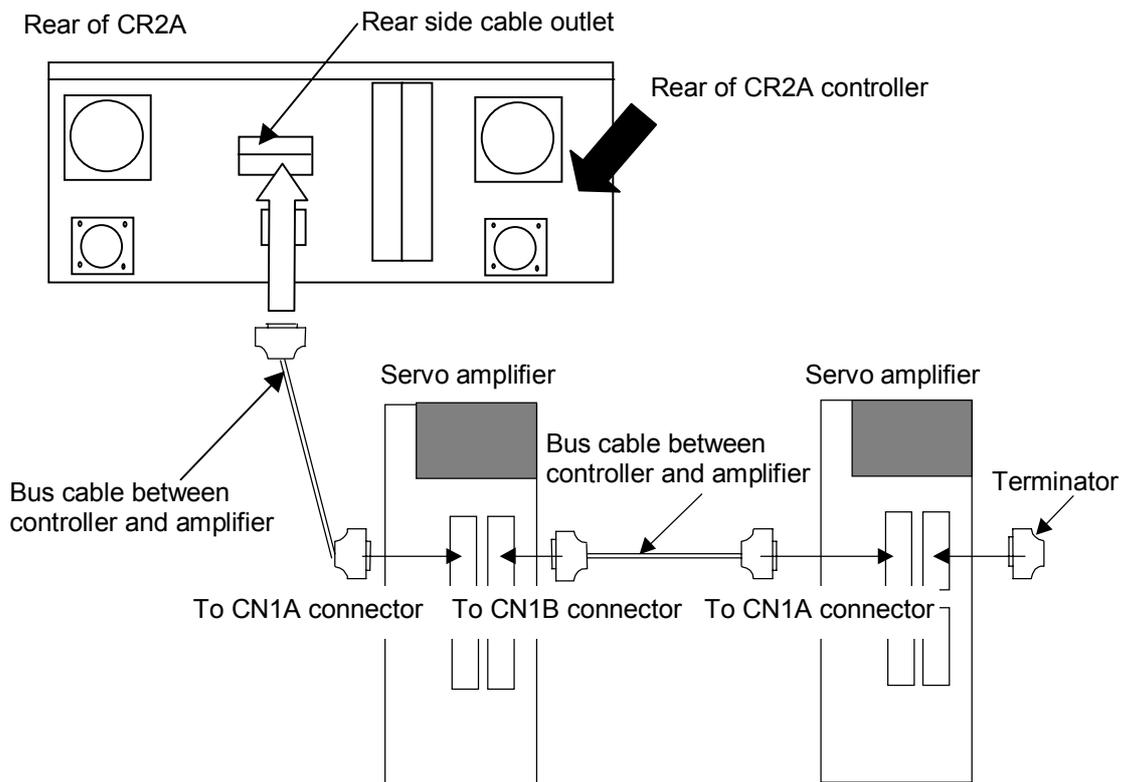
Fig. 5.2.3 Connecting the CR2A Controller and the Servo Amplifier
