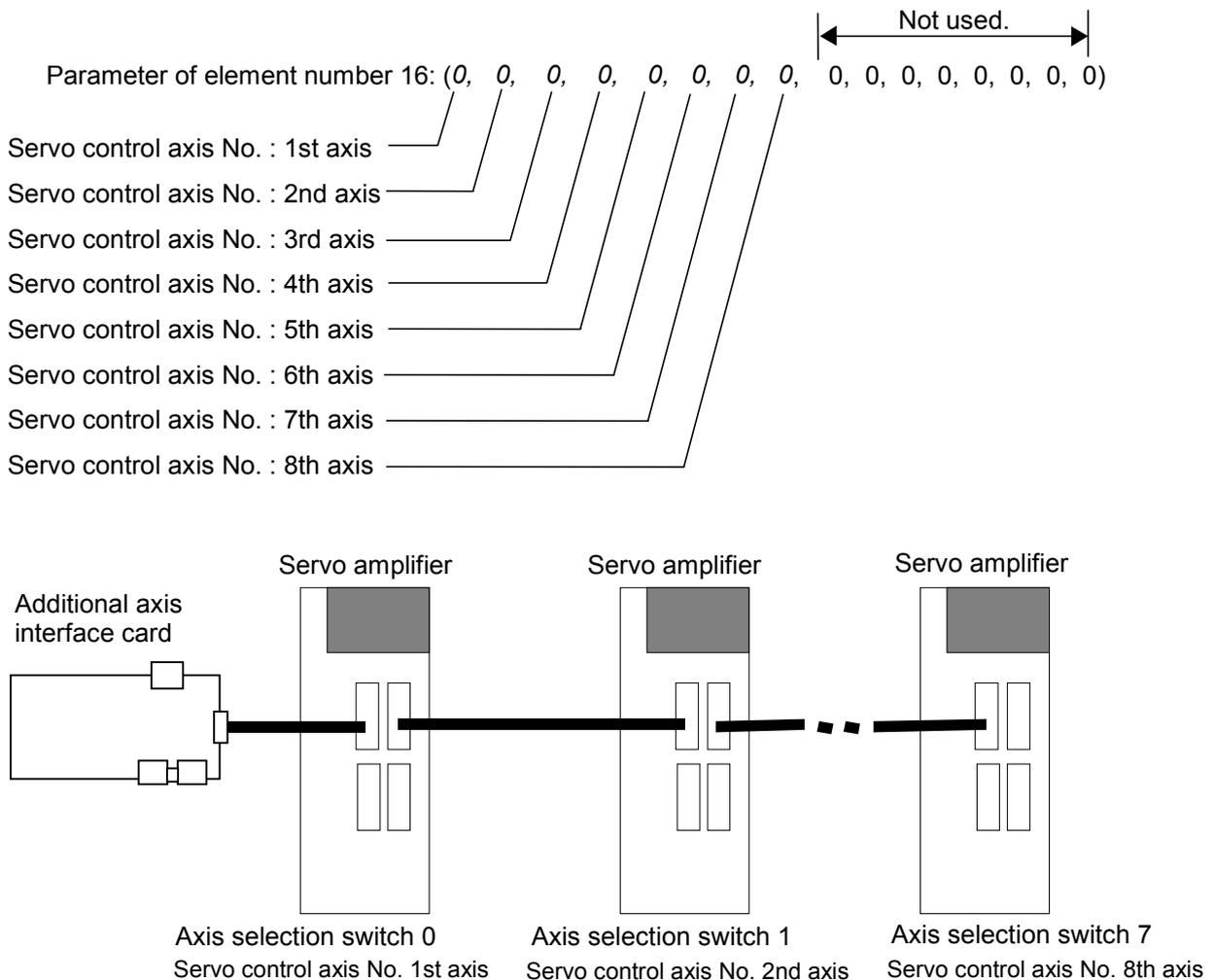
Fig. 7.1.1 Control No. and parameter element of servo
