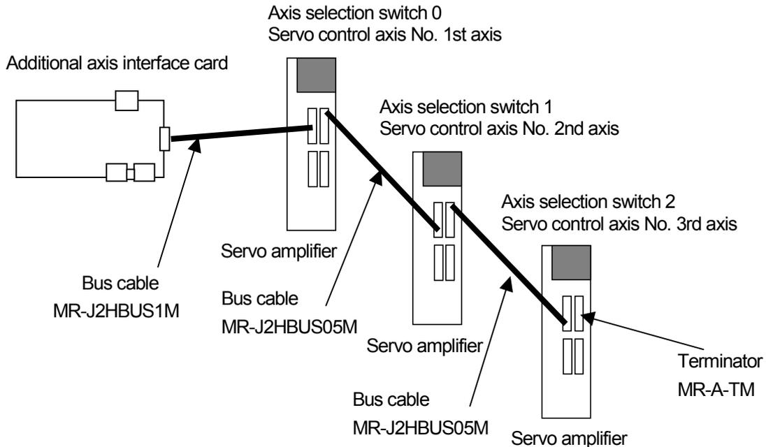
Fig. 8.7.5 Connection of controller and servo amplifier
