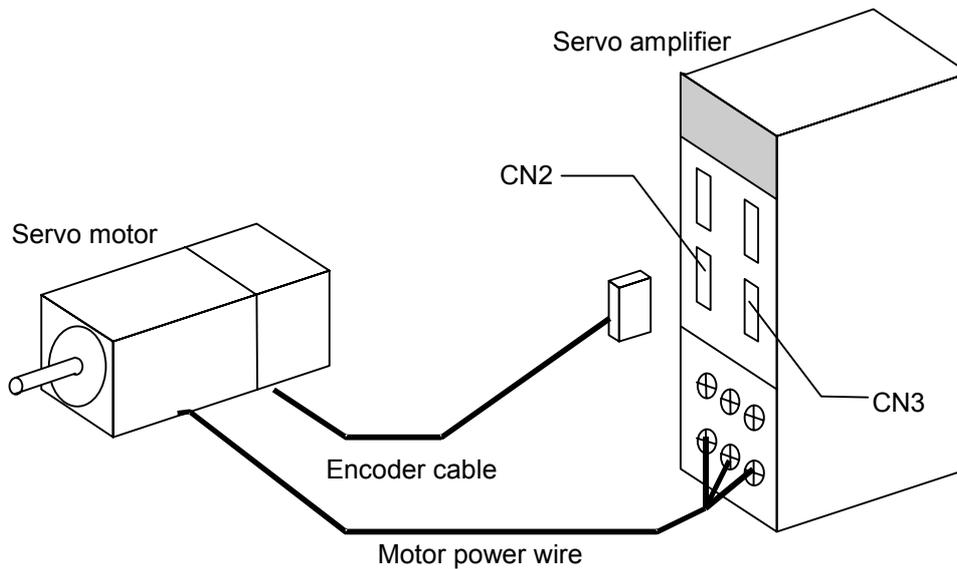
Fig. 5.4.1 Connection example of servo amplifier and servomotor
