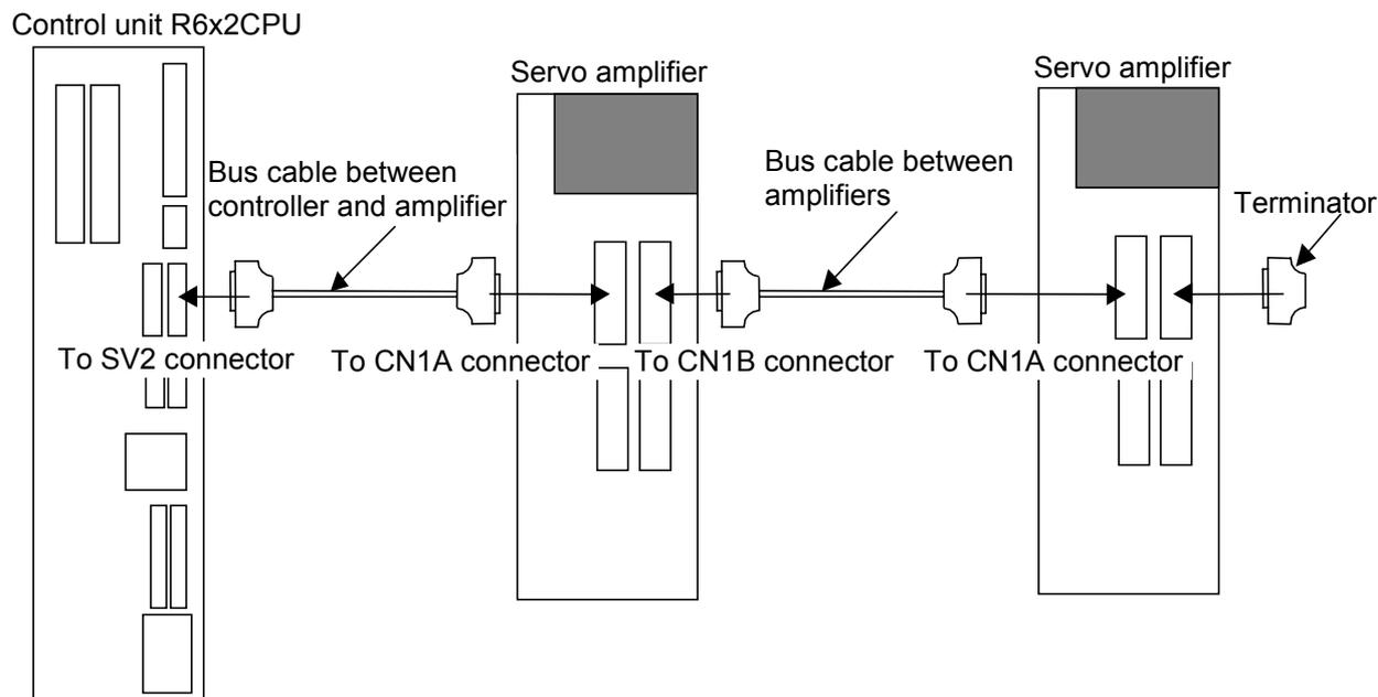
Fig. 5.3.2 Connection of Controller and Servo Amplifiers (CR2/CR4/CR8)
