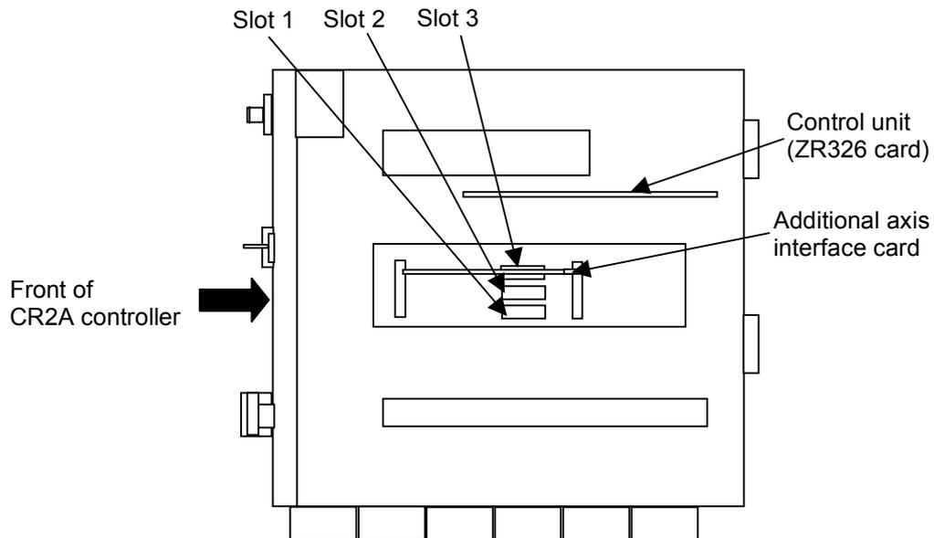
Fig. 5.2.1 Inside the CR2A controller (top side)
