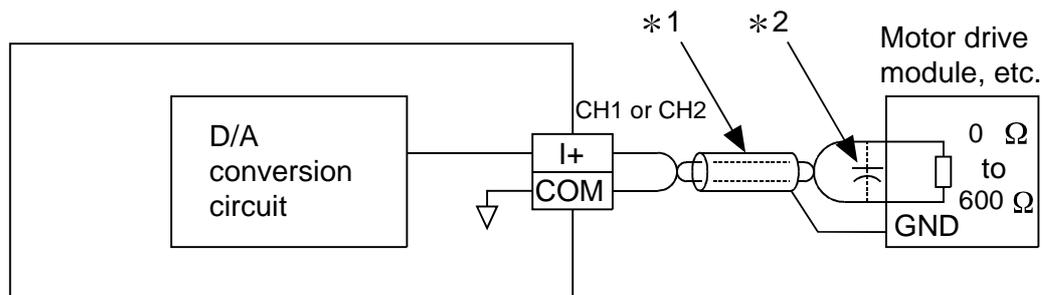
\*1 Use a two-core twisted shield line for the power cable.
