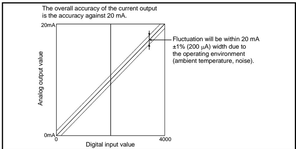
Fig. 3.4 Overall accuracy of current output characteristic
