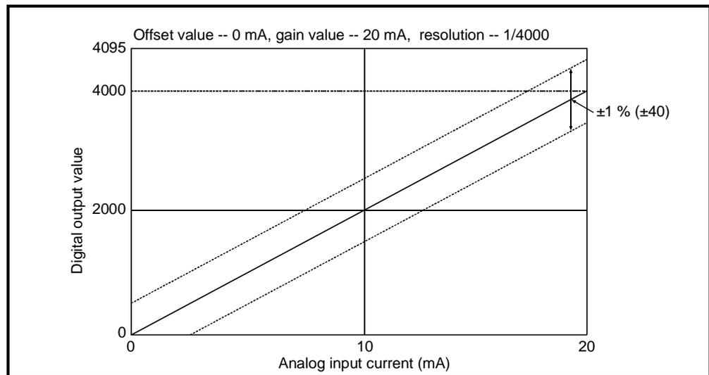
Fig. 3.8 Overall accuracy of current input characteristic
