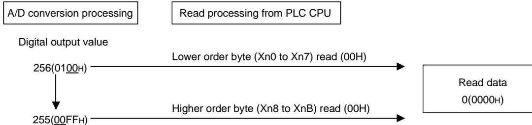
The read digital output value is compared every scan with the digital output value read at the previous scan to update only normal data. An example of a program to read a digital output value converted from analog on Channel 3 is shown below.
