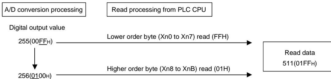
Example 2) When a digital output value is read from the PLC CPU during A/D conversion processing (during borrow occurrence) of the A1S66ADA
