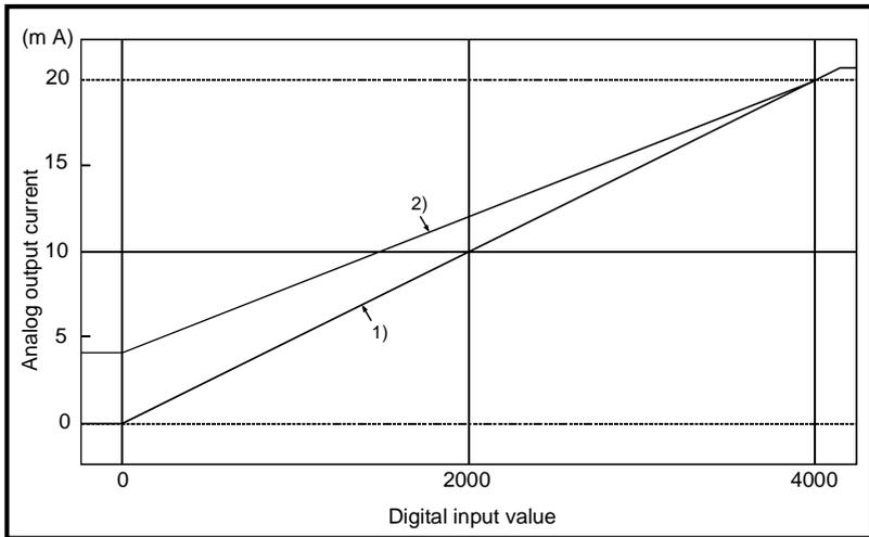
The I/O conversion characteristic when the off set value and gain value are set, as shown in the table below, is shown in the figure at left.
