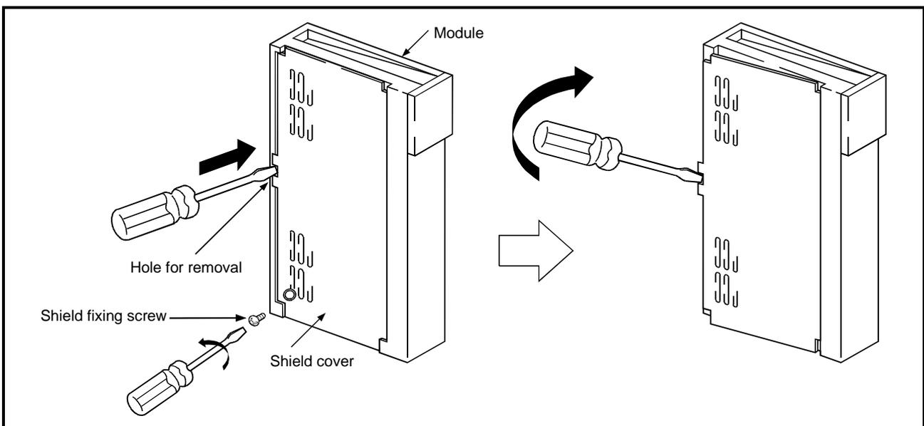
To remove the shield cover from the module, remove the shield fixing screw first and install the tip of a flat-tip screwdriver into the removal hole as shown in the figure, then move the screwdriver towards the rear of the module to separate the clip from the removal hole and remove the cover.
