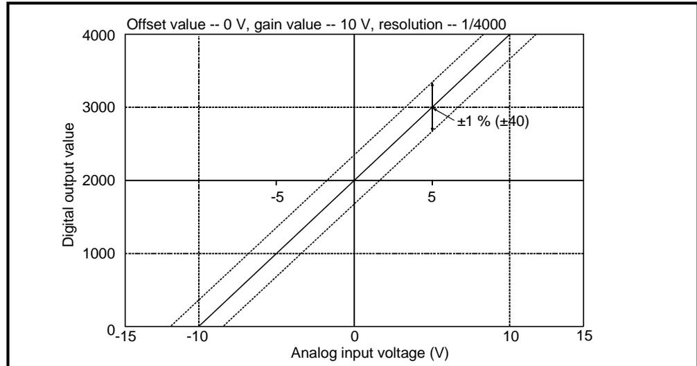
Fig. 3.7 Overall accuracy of voltage input characteristic
