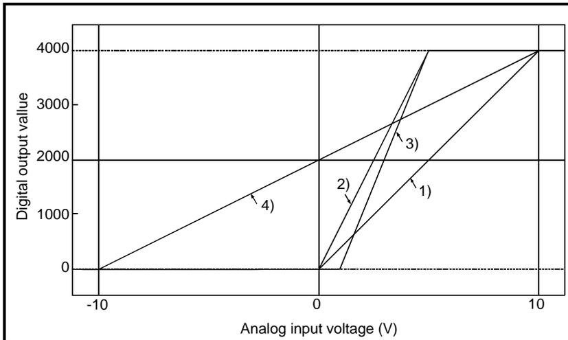
The voltage input characteristic when the offset value and gain value are set as shown in the table below, is shown in the figure.
