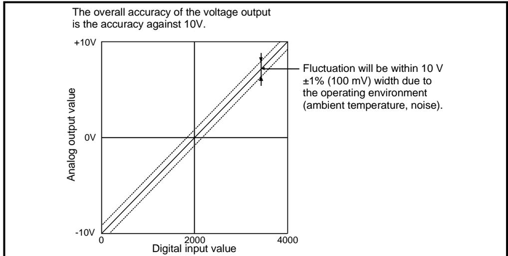
Fig. 3.3 Overall accuracy of voltage output characteristics
