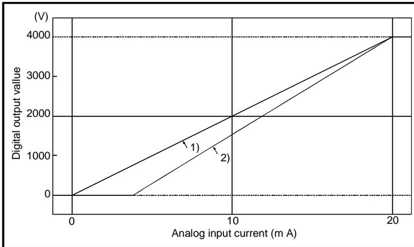
The current input characteristic when the offset value and gain value are set as shown in the table below is shown in the figure at left.
